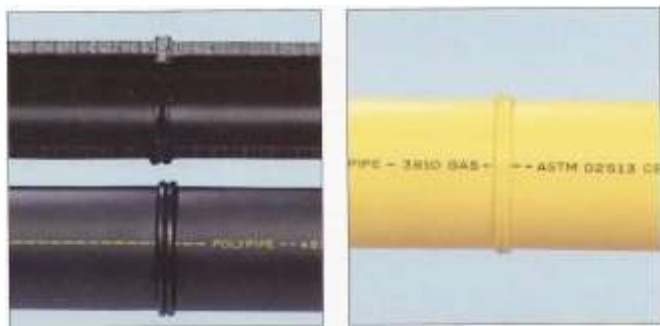
Proper alignment and double roll-back bead.
