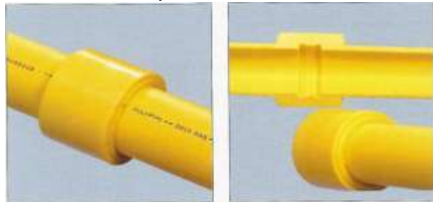
Proper alignment and stab depth. Melt bead flattened due to cold ring. No gaps or voids.
